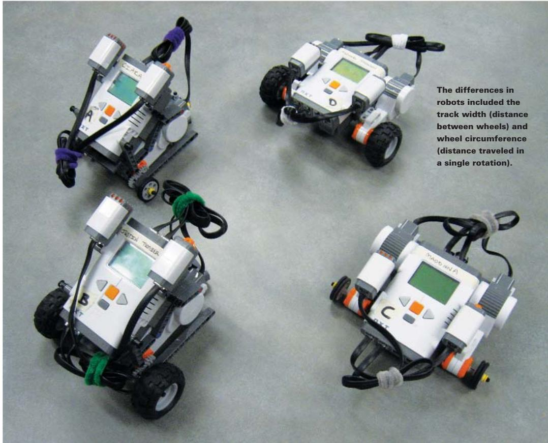
The differences in robots included the track width (distance between wheels) and wheel circumference (distance traveled in a single rotation).
